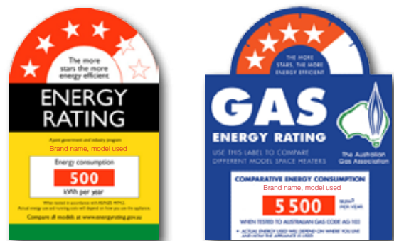
Energy rating labels allow you to compare the energy efficiency and energy consumption of some electric and gas appliances.
