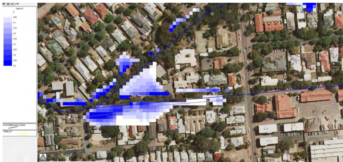
Figure B: Residual flood extent along Glen Osmond Creek downstream of King William Road (mitigation case / 100 year ARI)
