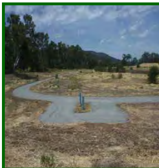
Monitoring Bore in the landfill
