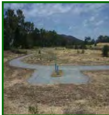
Monitoring Bore in the landfill
